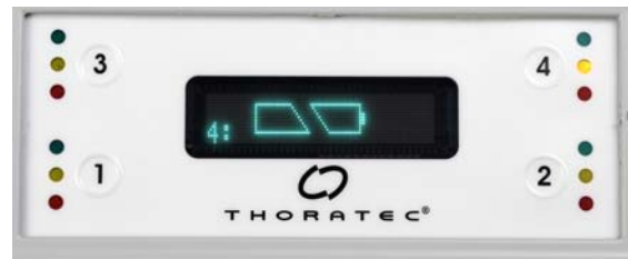
Figure 3.80 Calibration Status Screen Indicating that Battery in Pocket 4 is Being Calibrated
