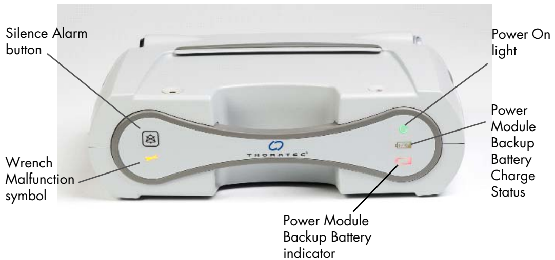
Figure 7.4 Alarm Indicators on Front of Power Module
