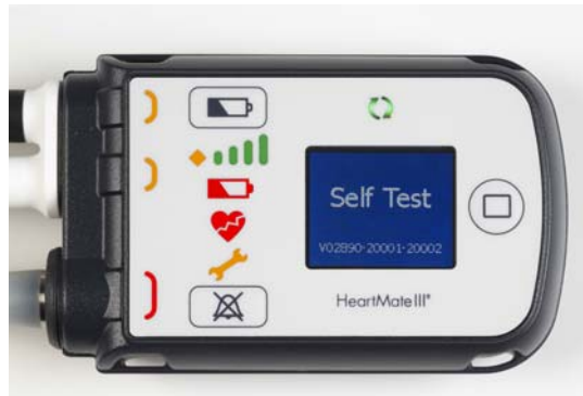
Figure 2.17 User Interface During System Controller Self Test
