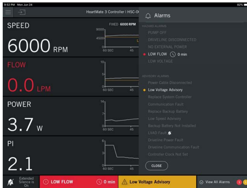
Figure 4.45 Alarms Panel with Multiple Active Alarms
