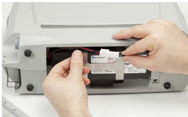
Figure 3.30 Gently Pull the Wires and Connectors Away
