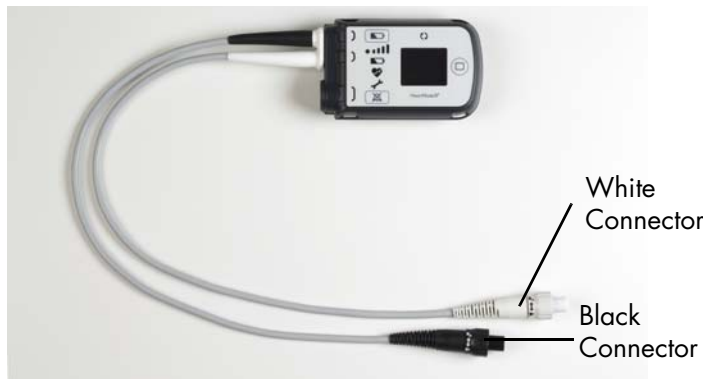
Figure 3.50 System Controller Power Cable Connectors
