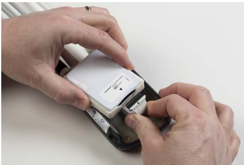
Figure 5.53 Align the Arrow on the Cable with the Arrow on the Battery
