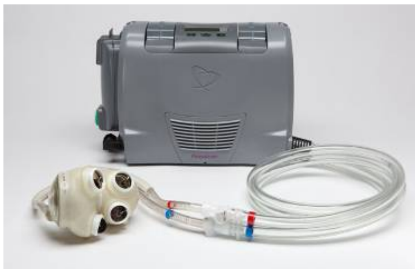
Figure 1-3 – Freedom Driver with Attached Power Adaptor and Drivelines Connected to the Cannulae of a TAH-t
