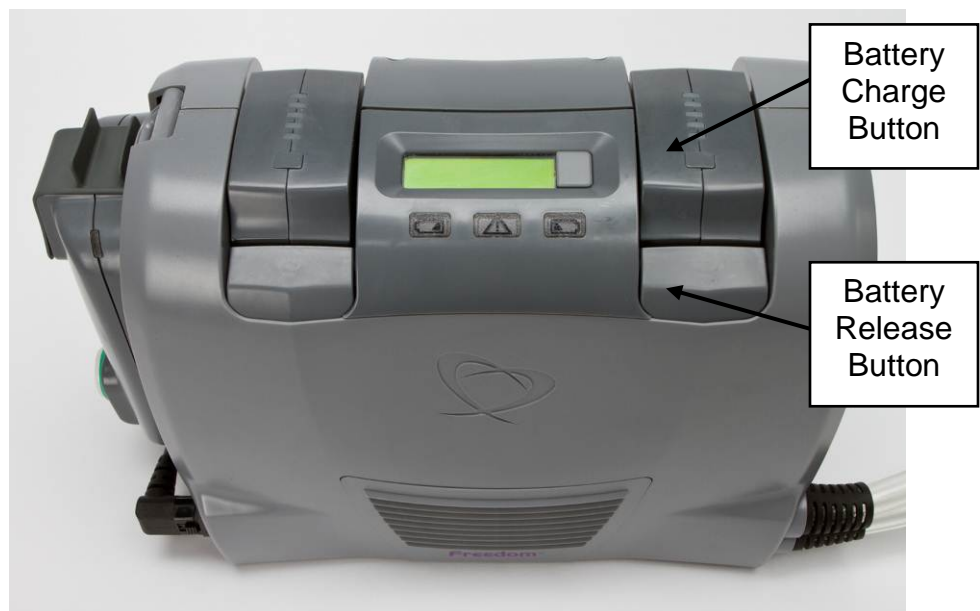
Figure 6-7 Correct Onboard Battery Insertion into Battery Well
