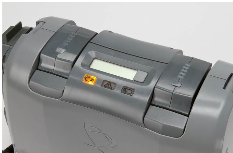
Figure 10-1 – Illuminated Flashing Yellow Battery Alarm Light
