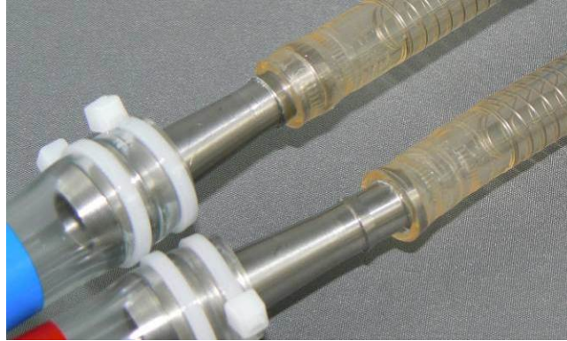
Figure 12-3 - Metal Hose Barb Connectors Loosened, But Still Connected, to the Cannulae
