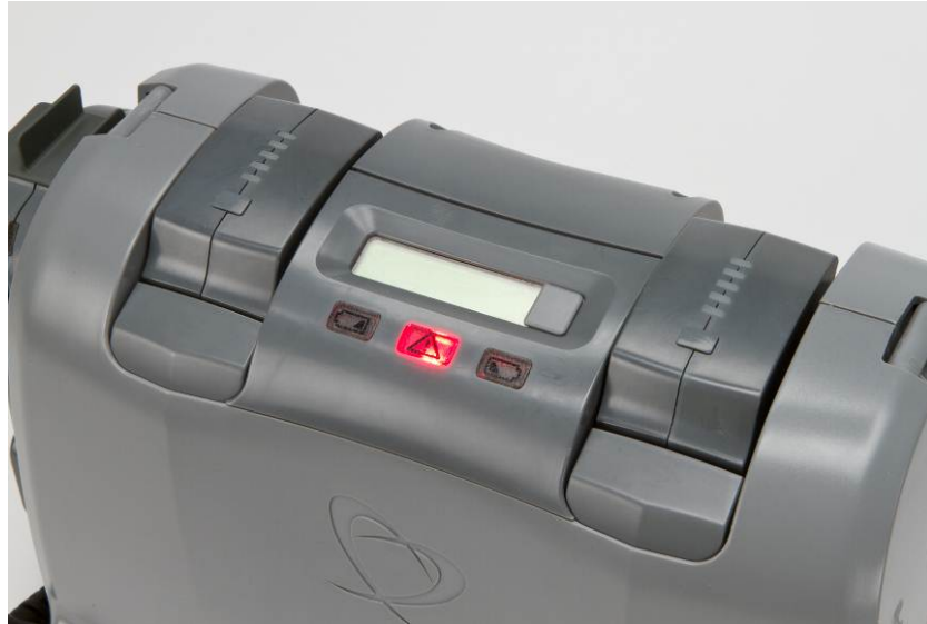
Figure 10-2 – Illuminated Flashing Red Temperature Alarm Light
