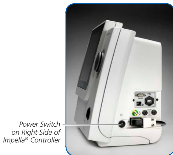
Figure 5.1 Automated Impella Controller Power Switch
