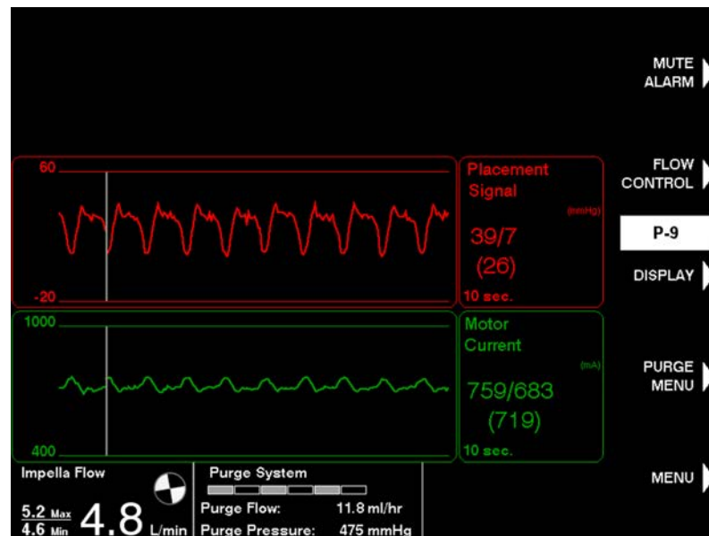
Figure 5.47 Confirming Placement on the Placement Signal Screen
