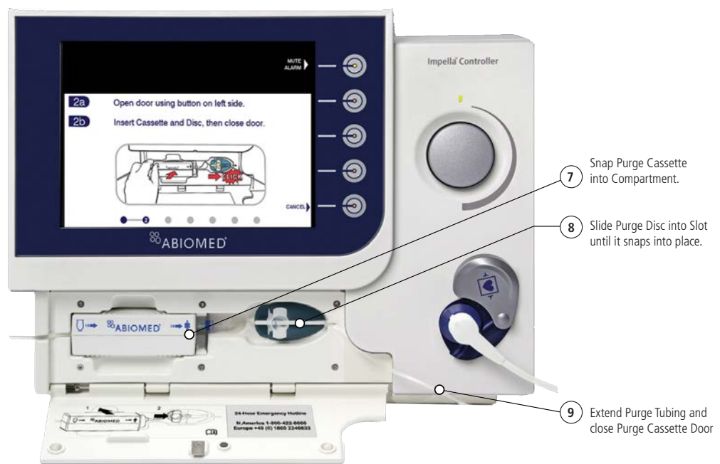
Figure 5.4 Inserting Purge Cassette into Automated Impella Controller
